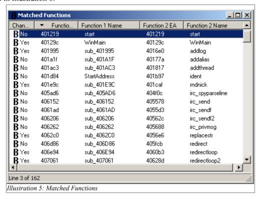
The first option, "Port", copies all sorts of comments and function names from the first file to the second one. How exactly this works can be configured in the BinDiff Options dialog. It's important to note at this point that this option will port the comments and names of all functions from one file to the other, not just the name and comments the selected function.
